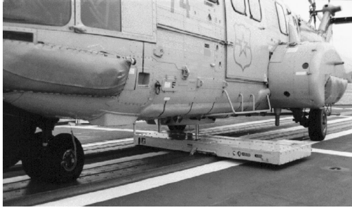
Fig. 1 ITI ASIST aircraft handling system (photo courtesy of ITI).
